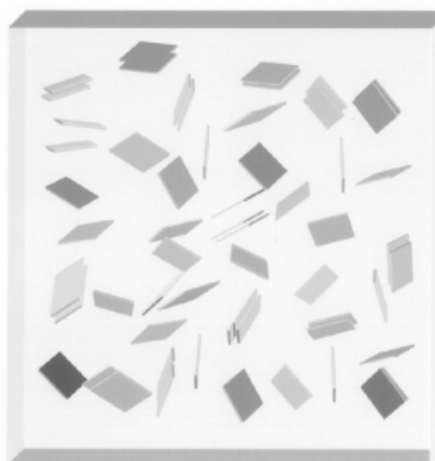
Figure 6 Clay dispersion in the epoxy/clay nanocomposites.
